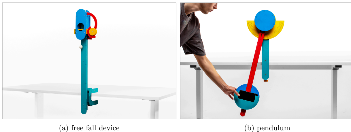
Figure 1: the devices for studying free fall and the pendulum.
