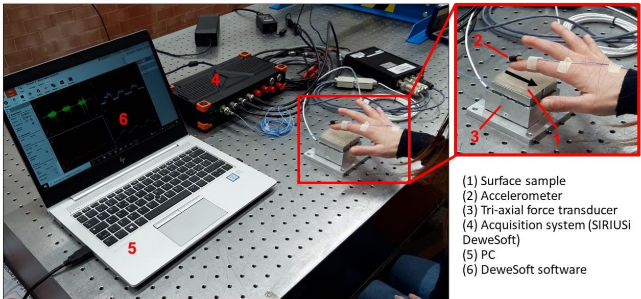
Figure 12: Active touch test bench for measurement of tactile mechanical stimuli.
