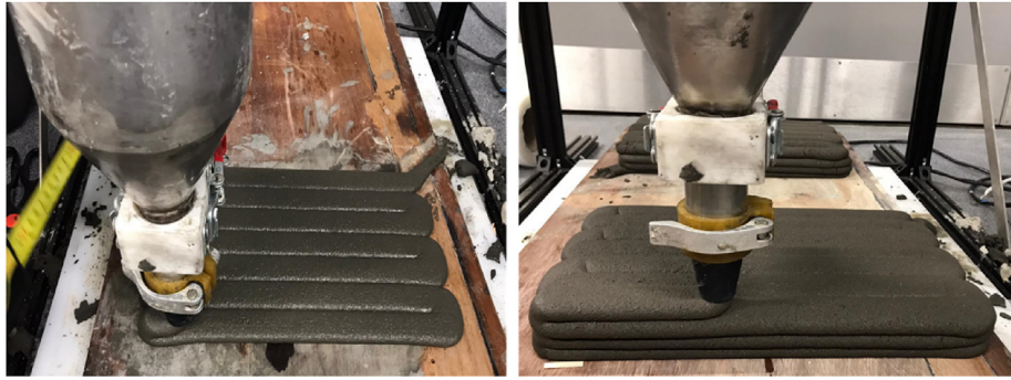
Fig. 9 – 3D printing of rubberized alkali-activated composites (100RP mix is reported in the photographs).
