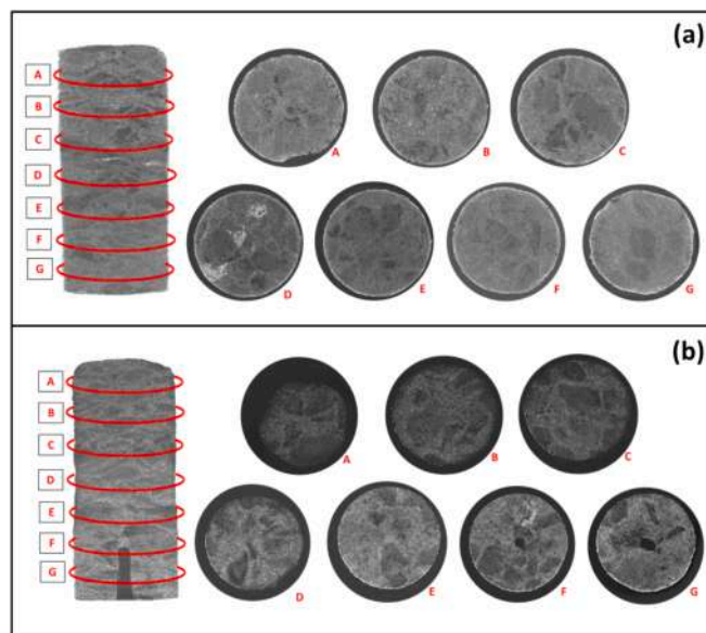
Fig. 11. XRM scan for virgin sample 160/10 (a) and charred sample 160/10(b).
