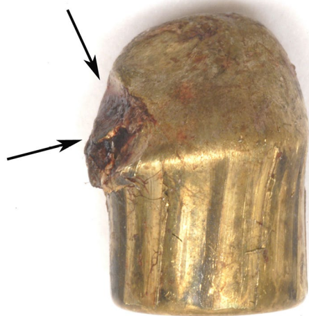
Fig. 3 Cal. 9-mm bullet retrieved during crime scene investigation, characterized by a deformation produced by the contact with the metal wire fence (upper arrow) and the glass (lower arrow)
