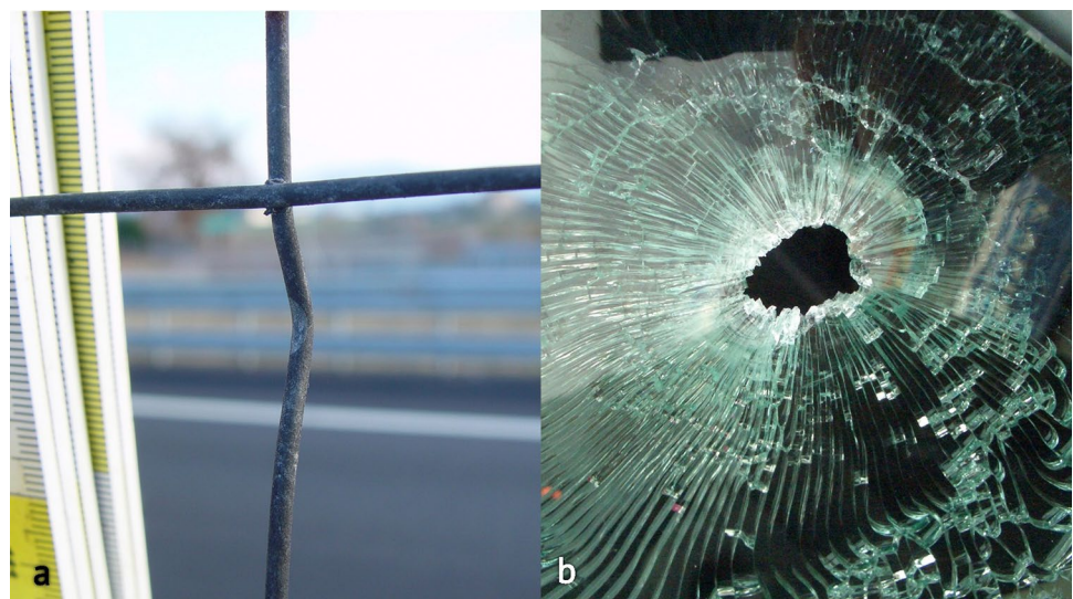
Fig. 1 Case 1 intermediate targets. a First intermediate target: the wire fence dividing the two carriageways. Interaction with the bullet caused a “watermelon slice”-like deformation of the metal and subsequent ricochet from the original trajectory. b Second intermediate target: glass of the rear window. Note the shape of the hole which accurately represents the lateral projection of the bullet
