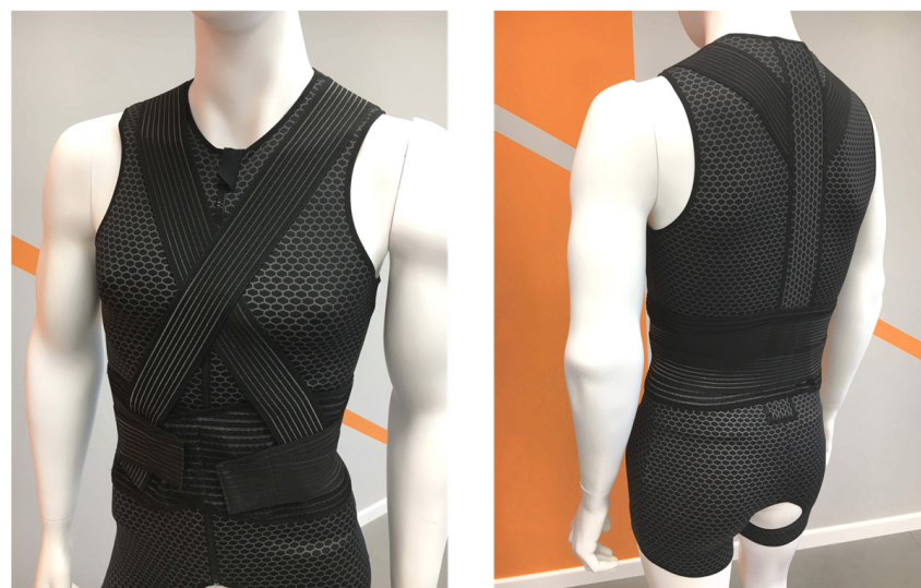
Figure 1. Textile module made of Lycra fabric woven with carbon thread; soft passive exoskeleton.
