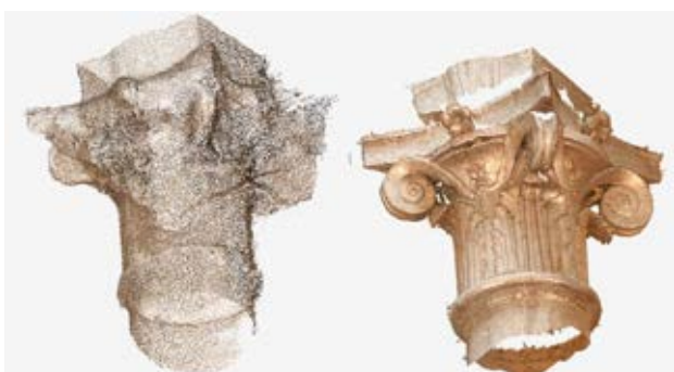
Figure 10. The difference in density between the capital represented by the entire courtyard point cloud (69,000 points) using 15-mm optics and the capital extracted with detail photos (4,156,625) taken with 70-mm optics
