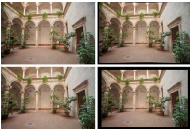
Figure 5. Upper left: An original photographic image from the campaign. Upper right: Photo corrected by PhotoModeler. Lower left: Photo corrected by Photoscan. Lower right: The photo corrected with Photoscan was scaled and aligned with the PhotoModeler correction and superimposed with 50% opacity.
