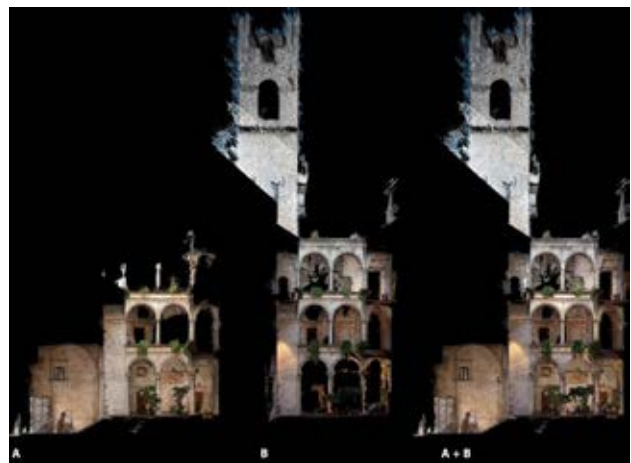
Figure 17. Sections of the point cloud in orthographic projection obtained from the two photography campaigns. A: first campaign, B: second campaign, A+B: overlay of the two campaigns
