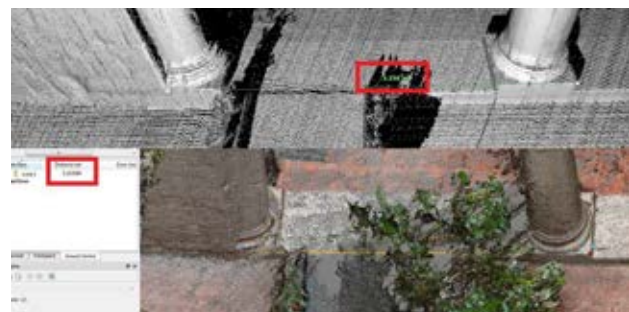
Figure 8. Sample measurements to check the scaling and orientation of the point cloud in Photoscan
