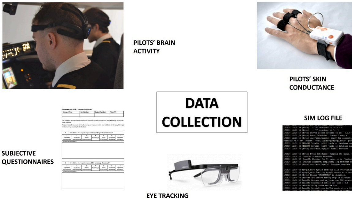
Fig. 3. Pilots' behavioural, subjective and neurophysiological data were acquired together with the simulator log - files during the entire flight simulation and WVEs.
