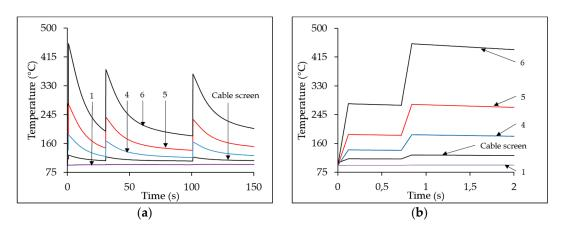
**Figure 5.** (a) Thermal transients in SCJ (cases 1, 4, 5, and 6) and in the cable screen (case 3).  $I_F = 3$  kA, UC A1. (b) Zoom of (a) in the timeframe from 0 s to 2 s.
