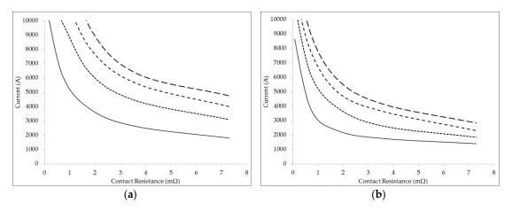
**Figure 9.** Fault current values causing SCJ heating up to the maximum tolerable temperature, as a function of joint CR. Four different maximum tolerable temperature are considered: 250 °C (solid line), 500 °C (dotted line), 750 °C (short-dashed line), and 1000 °C (long-dashed line). (**a**) 120 ms fault clearing time (UC A1); (**b**) 320 ms fault clearing time (UC B1).
