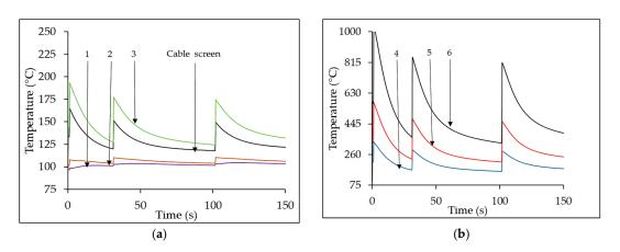
Figure 6. Thermal transients for  $I_F$  = 3 kA (UC B2). (a) Cases 1, 2, and 3; (b) Cases 4, 5, and 6.
