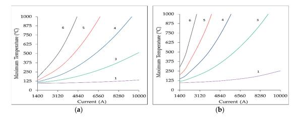
**Figure 4.** Maximum temperature calculated for short circuit currents cleared in 120 ms (**a**) and 320 ms (**b**); different CR values are simulated, as defined in Table 6.
