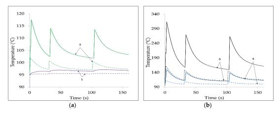
**Figure 7.** Thermal transients along SCJ,  $I_F = 800$  A; fault clearing times: 1070 ms (solid line) and 320 ms (dashed line). (a) Cases 1 and 3; (b) Cases 4 and 6.
