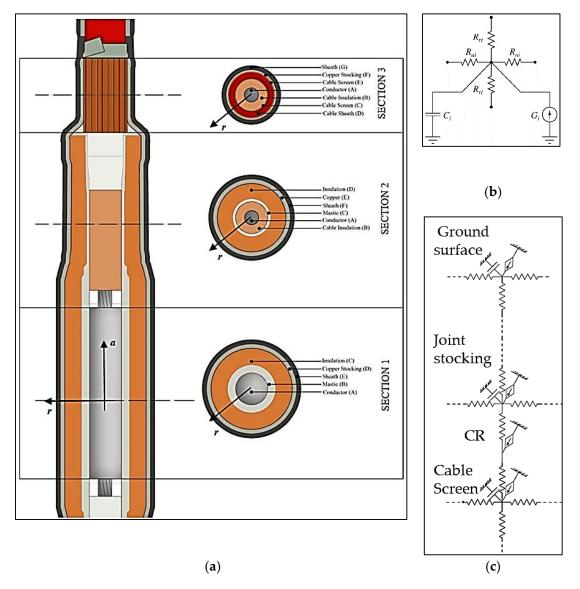
**Figure 1.** (a) Simulated cold-shrinkable joint (the cylindrical coordinate system used in the model is also shown), extracted from [14]; (b) Equivalent electrical circuit corresponding to each layer of the cable; (c) Detail of the equivalent network representing the contact resistance (CR).
