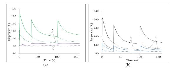
**Figure 8.** Thermal transients along SCJ,  $I_F = 1400$  A; fault clearing times: 320 ms (solid line) and 120 ms (dashed line). (a) Cases 1 and 3; (b) Cases 4 and 6.
