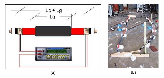
**Figure 2.** (a) Outline of the experimental setup for CR measurements; (b) Laboratory setup for the tests [19].
