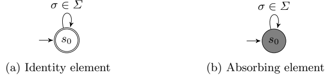
Fig. 4: Finite state automata acting as identity element and absorbing element for the automata cross-product operation.
