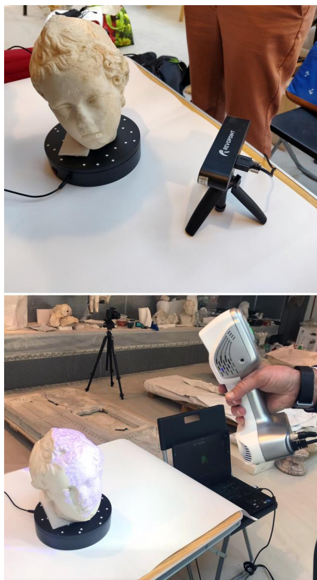
Figure 6. Indoor acquisition set with roundtable: on the top POP 3D scanner, on the bottom iReal 2S scanner.
