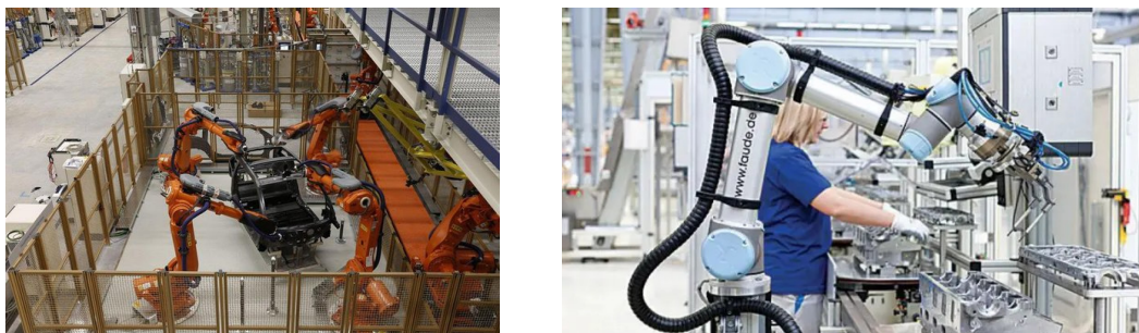
Figure 1.1. Robot manipulators operating in an industrial environment. Note how in the traditional setting (left) robots are placed in a cage where humans are not allowed in during operation, while cobots (right) can safely operate alongside humans.
