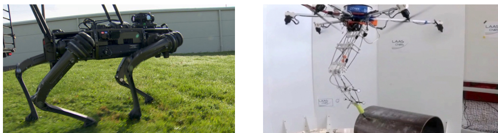
Figure 1.3. Examples of more complex articulated mobile robots. A quadruped robot equipped with a array of sensors for patrolling (left) and a fully actuated aerial manipulator (right).
