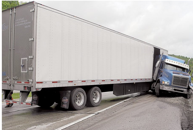
Figure 5.1. Tractor-Trailer vehicle having crashed after jackknifing.
