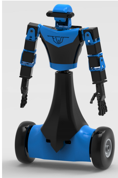
Figure 4.1. ALTER-EGO, a prototype WIP robot developed at the University of Pisa [72].
