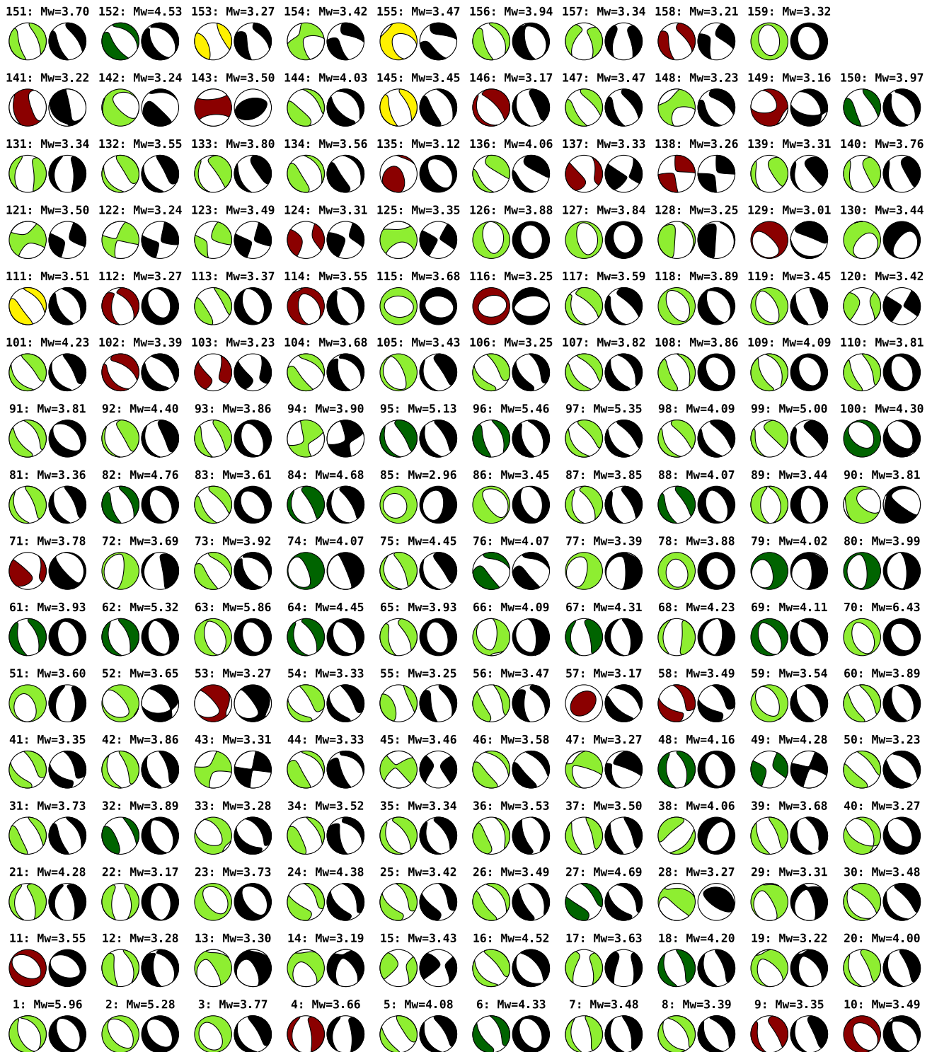
Figure 2. Catalog of the retrieved solutions for the 159 3D Centroid Moment Tensor (CMT-3D) events. The beachballs on the left are colored according to \tau definition, while the black beachballs on the right are the time domain moment tensor (TDMT) input solutions. M_w values are those of the CMT-3D solutions.
