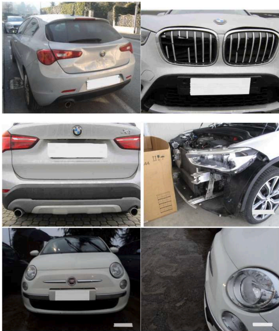
Fig. 3. Damages suffered from the vehicles involved in a multiple rear-end collision.
