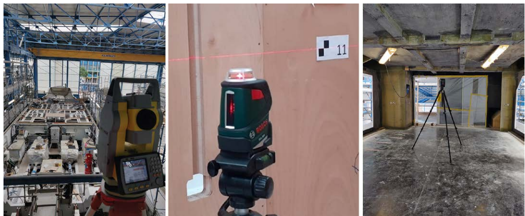
Fig. 4. Phases of boat acquisition through total station, laser level and 3D laser scanner. Elaboration by the authors.
