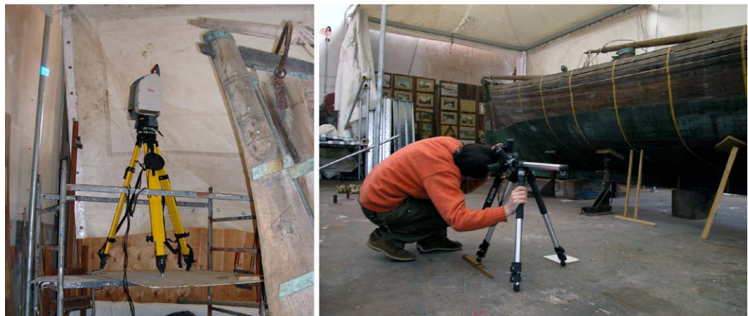
Fig. 2. Phases of acquisition of the boat's surfaces: on the left, with a 3D laser scanner; on the right, with a photogrammetric technique. Elaboration by the authors.
