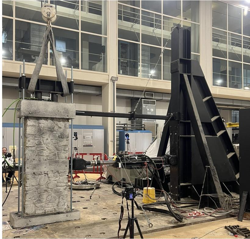
Figure 6.3: Set-up of the Sheppard test
