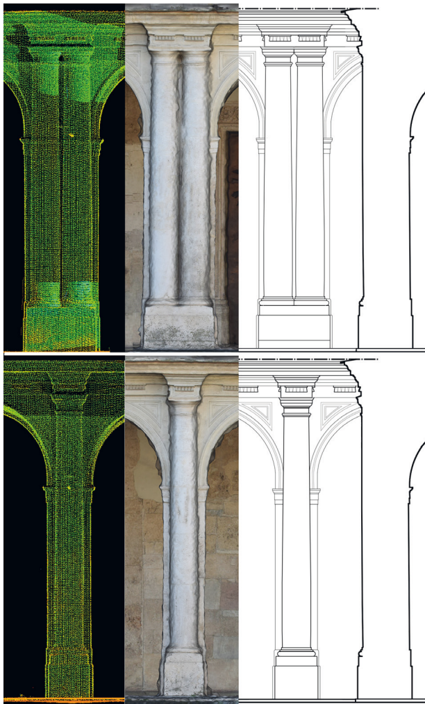
Figure 5. Construction of real 3D/2D models of the half column and the binate column.
