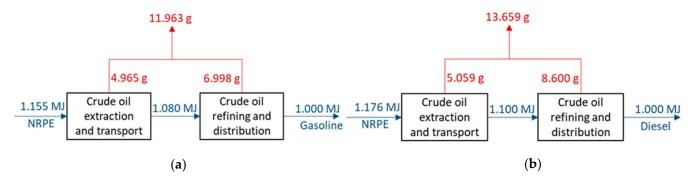
Figure 3. WTT analysis for gasoline (a) and diesel (b) [12].
