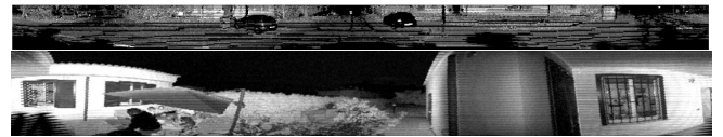
Fig. 3: Projection of the KITTI LiDAR point cloud into an image plane (up), projection of our LiDAR into an image plane (down). The many holes of the up image due to uneven distribution of the LiDAR beams and calibration issues make the KITTI LiDAR image unusable for computer vision tasks.
