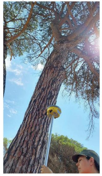
Figure 4. The survey with the Geomax receiver where the tree cover issue is evident
