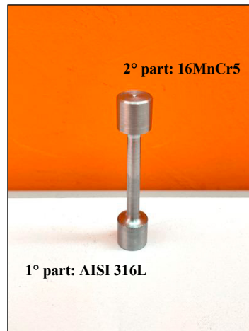
Fig. 2. Multi-material tensile specimen: AISI 316L and 16MnCr5 steel.
