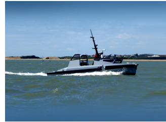
Figure 2: An example of ASV: Thales Halcyon ASV.
