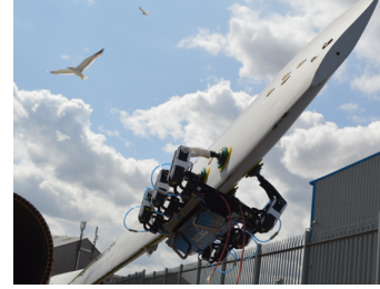
Figure 4: An example of crawling robot: BladeBUG robot.
