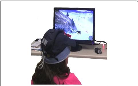
**Fig. 3** A training session with ENLAZA. The user has a wired IMU attached to a baseball cap and plays the game Extreme Tux Racer
