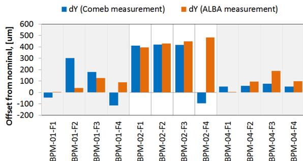
Figure 9: Fiducial position deviations from nominal in Y.
