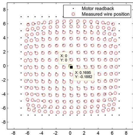
(a) BPM response map measured by wire scanning within  $\pm 7$  mm. The central point corresponds to the wire homing position (0, 0). Its electrode readings correspond to the mechanical offset of the BPM.
