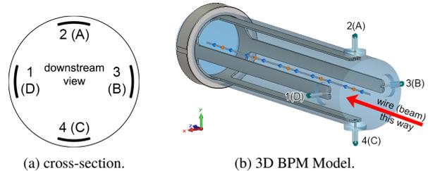
Figure 1: Naming convention and 3D BPM Model.
