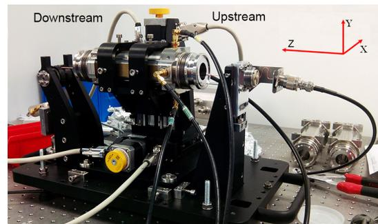
Figure 2: Photo of the BPM and the test bench in the lab.
