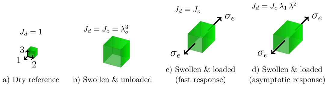
FIG. 3. From left to right: (a) dry state; (b) free-swollen state; (c) fast response state under swelling and loading; (d) asymptotic state under swelling and loading. For a gel with  $G = 0.1$  MPa,  $RT/\Omega = 40$  MPa,  $\chi = 0.2$ , under a traction  $\sigma_e = 0.1$  MPa, we have:  $J_o = 18.5$ ,  $J_d \approx 23$ . Plots are in scale.
