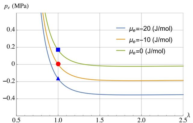
FIG. 2. Pressure–stroke curves  $p_e(\lambda, \mu_e, \lambda_o)$  for three values of  $\mu_e$  with  $\lambda_o = 2$ , corresponding to  $\mu_o = -10$  J/mol. When  $\mu_e < \mu_o$  ( $\mu_e > \mu_o$ ) the corresponding blocking pressure is determined on the vertical axis  $\lambda = 1$  in correspondence of the blue triangle (square) on the blue (green) curve.
