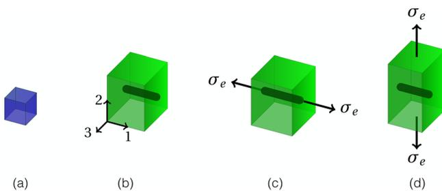
FIG. 6. From left to right: (a) dry state; (b) free-swollen state:  $\sigma_e = 0$ , and  $\mu_e = -10$  J/mol; (c) swollen with traction along the fiber:  $\sigma_e = 50$  kPa, and  $\mu_e = -10$  J/mol; (d) swollen with traction orthogonal to the fiber:  $\sigma_e = 50$  kPa, and  $\mu_e = -10$  J/mol.
