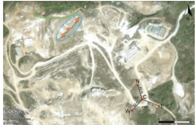
Fig. 2 - Satellite view showing the SNS array installed in the quarry district of Coreno Ausonio: the “reference wall” is shown by the green ellipse, the “reference quarry” by the blue ellipse and the blasts of known location by the red stars
