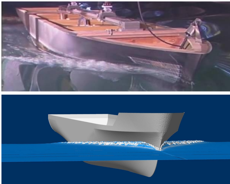
Figure 10.39.: Breaking bow wave during experiments at DGA- Hydrodynamics (top) and 3D view of the breaking bow wave in the SPH simulation (bottom plot), Fr = 0.328 .
