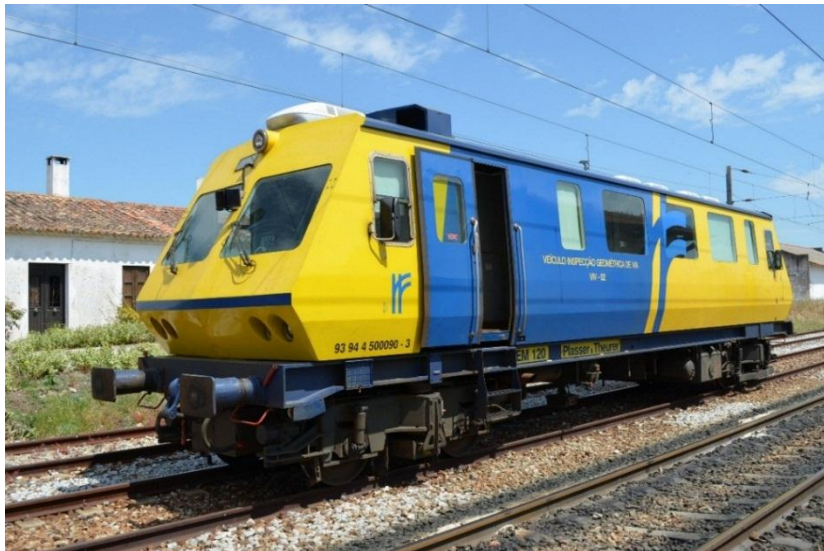
Figure 3.3 - EM120 diagnostic train
