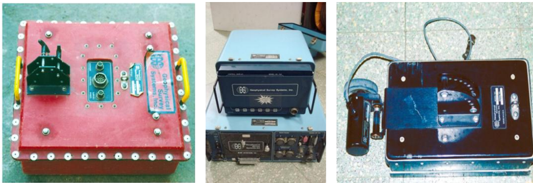
Figure 4.13 - GSSI system: SIR 10H (middle), 500 MHz (left) and 900MHz (right) ground-coupled antennas
