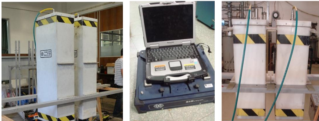
Figure 4.12 - GSSI system: 1 GHz (left) and 1.8 GHz (right) air-coupled antennas
