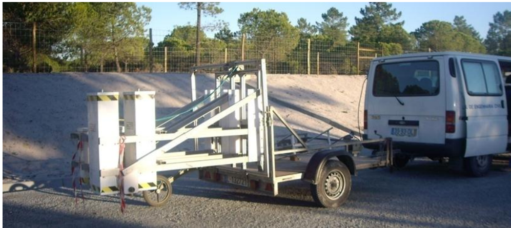
Figure 2.6 - LNEC's GSSI air-coupled antennas
