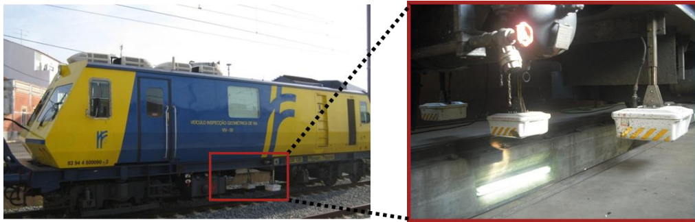
Figure 3.7 - Portuguese monitoring equipment: EM120 and GPR
