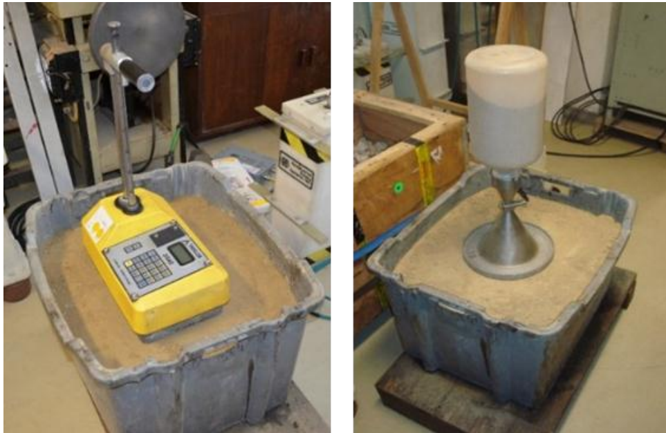
Figure 4.21 - Water content measurements: Troxler (left) and sand-cone density apparatus (right)
