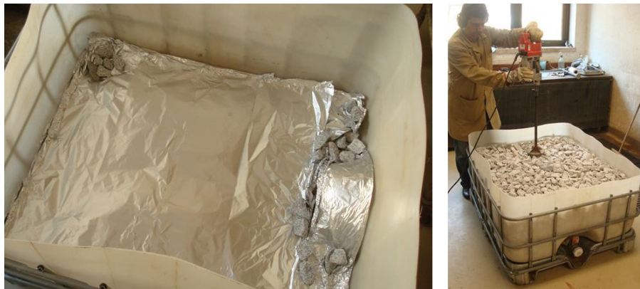
Figure 4.7 - Aluminium sheet placed on the bottom of the box (left) and ballast compaction (right)
