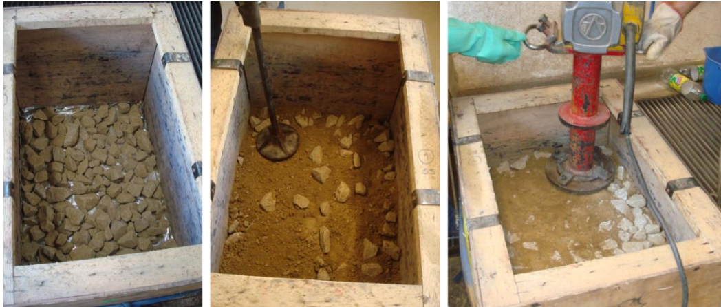
Figure 4.10 - Highly fouled ballast: phases of construction
