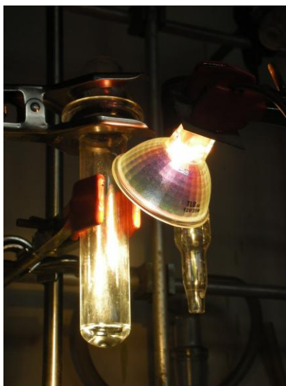
Figure 5.2.1: Photochemical functionalization of Si wafers in a Schlenk-line.
