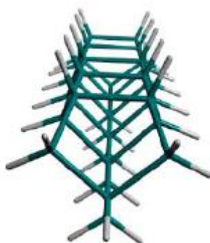
Figure 2.1.3: Si(100)-2x1 reconstruction, from DFT calculations.
