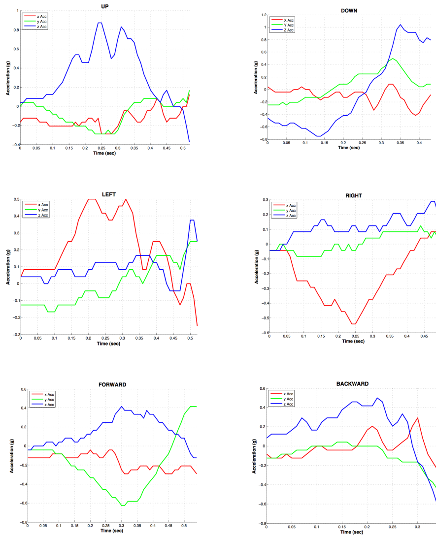
Figure 5.1: Examples of accelerometer data representing some gestures.
