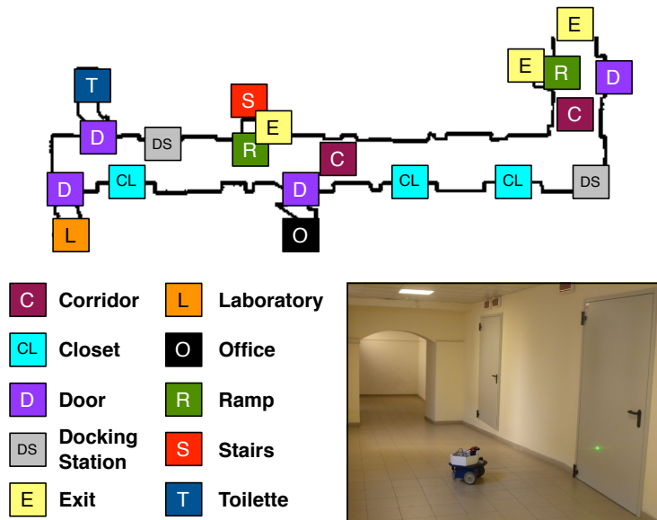
Figure 7.3: Output of the robot mapper through the semantic knowledge acquired by the operator for a surveillance scenario. Knowledge about structural elements and relevant elements is overlaid on the metric map built by the robot.
