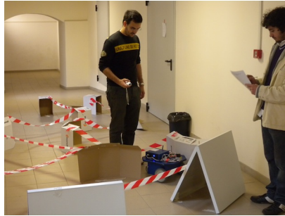
Figure 4.3: An operator controlling a wheeled robot with our tangible interface for teleoperation. Pitching down (up) the Wiimote device increases (decreases) the robot linear speed, while rolling left (right) the device corresponds to turning left (right) the robot.
