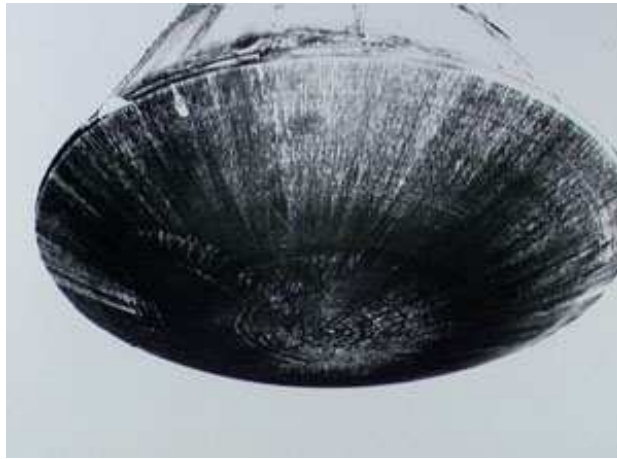
Figure 3: Mercury spacecraft ablative heat shield after recovery.
