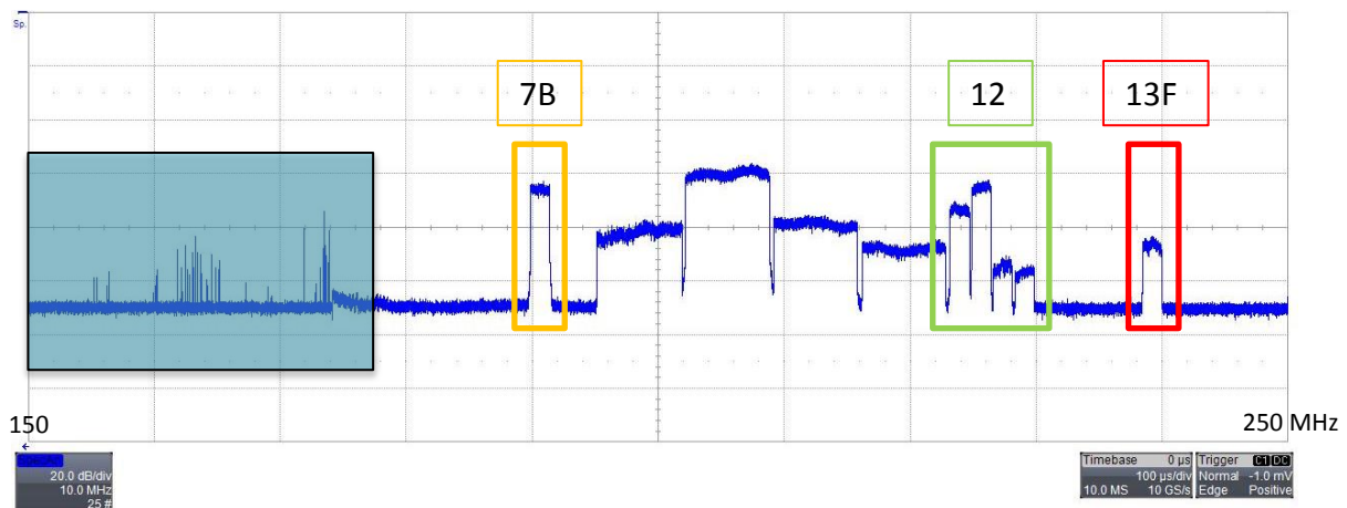
Figure 85 FM radio signal residuals after FM band filtering.
