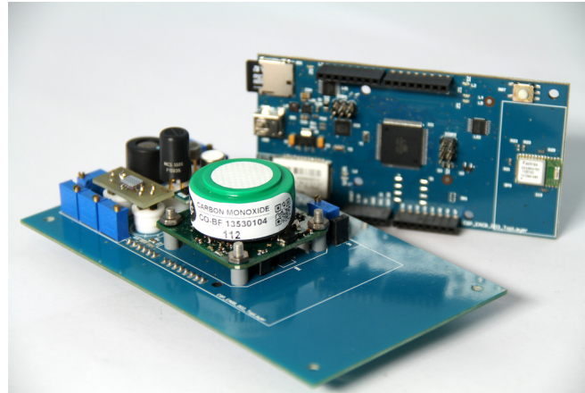
Fig 8. Sensing device. The two electronics boards of the sensor box with the gas sensors mounted on top of the sensor shield.
