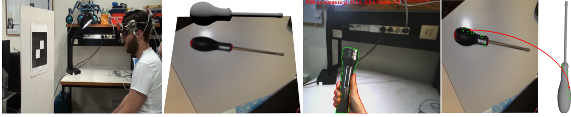
Fig. 2: First: GM calibration phase. Second: 3D model obtained from the tool silhouette. Third: segmented tool and hand. Forth: collected PORs back-projected on the model.
