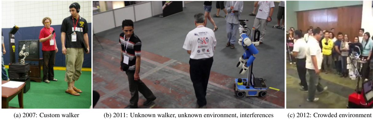
Figure 2: Evolution of 'Follow me' test. Starting with known guides in a known environment, the test is now conducted with unknown guides in an unknown environment with several interferences along the route.
