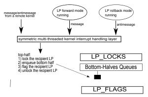
Figure 2: The top/bottom-halves architecture.
