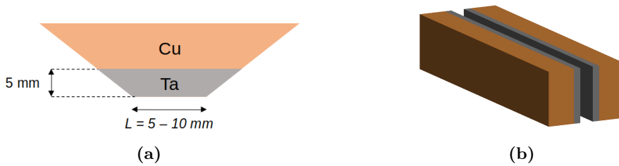
Figure 4.6. (a) Schematic layout of a jaw of a SuperKEKB-type collimator, consisting of a copper body with a short high- Z tip made of tantalum (Ta) or tungsten (W), typically 5–10 mm in length. (b) View of the CollimatorTipJaw element ("jcoltip") implemented in BDSIM, used to realistically reproduce the two-material structure of SuperKEKB-type collimators in simulation.
