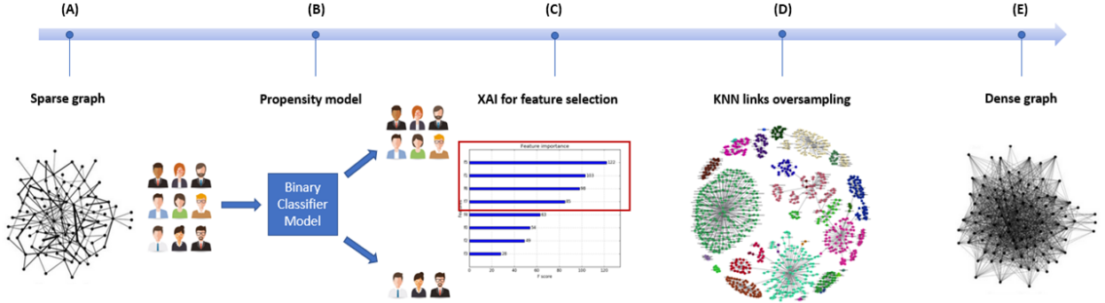
Figure 3.2: A schematic representation of the proposed framework for graph construction. (A) The initial sparse graph. (B) A propensity model is trained, then (C) Shapley values are computed to select the most representative features. (D) A bipartite graph is built using interaction data, with link augmentation for users and items. Finally, a dense graph (E) is obtained.
