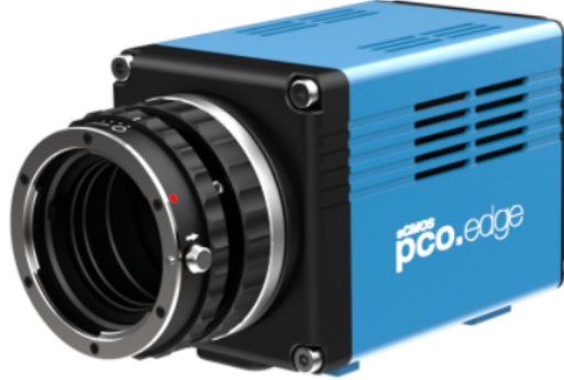
Figure 5.7: Photograph of the CCD camera used for the diagnostics. The camera features a pixel pitch of 6.5 \mu m , a resolution of [2560 \times 2160] pixels, and a dynamic range of 30000:1 [67].
