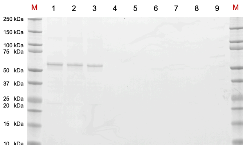
Figure 36. SDS–PAGE analysis of TB002 recovery after 0.22 \mu\text{m} sterile filtration. Lane M: molecular weight marker; Lane 1: bulk material; Lane 2: bulk after UV sterilization (2h, RT); Lane 3: bulk after room temperature incubation (RT); Lane 4: cellulose acetate (CA) filter, CHROMACOL; Lane 5: nylon filter, CHEBIOS; Lane 6: cellulose acetate (CA) filter, ADVANTECK; Lane 7: PES filter, Sartorius; Lane 8: cellulose acetate (CA) filter, VWR; Lane 9: PES filter, VWR. The gel confirms that significant protein loss occurs when TB002 is passed through syringe filters, regardless of membrane type.
