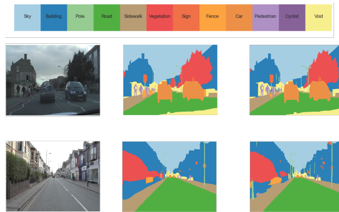
Figure 4.1: Semantic Segmentation: original image, original annotation (ground truth) and prediction of the model [48]
