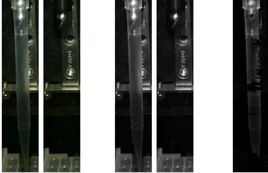
Figure 4.2: Example of pre-processing up to the subtraction step for a long tip. The figure displays the scene image and the corresponding background before grayscale conversion (left), after grayscale conversion (center), and the resulting subtracted image (right).
