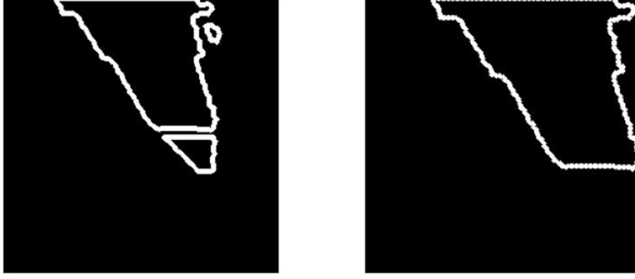
Figure 4.8: Example of a contour image obtained after pre-processing (left) and its corresponding reconstruction using the first 8 Fourier descriptors (right) for a short tip.
