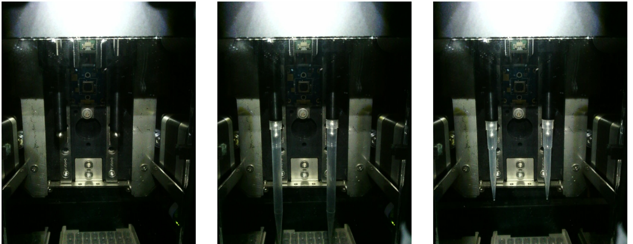
Figure 2.7: Example of image acquired by the machine vision system: before tip grip (left), after two 1000 \mu\text{l} tips grip (centre) and after two 200 \mu\text{l} tips grip (right).
