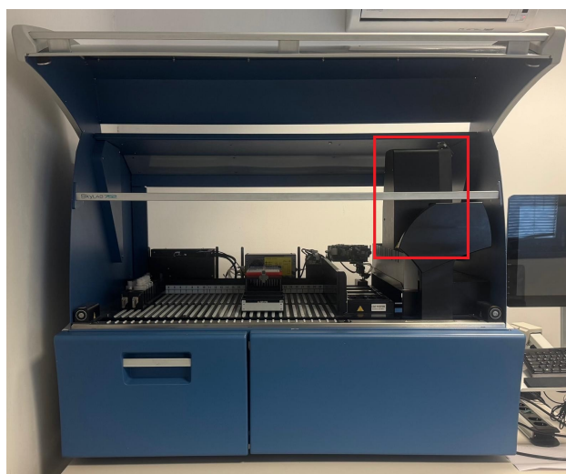
Figure 2.5: The IVD device in an open state. The red box highlights the pipetting system, which houses the monitoring system.
