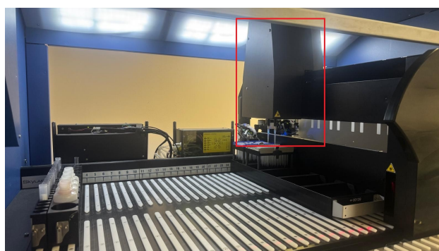
Figure 2.6: Internal view of the IVD device. The pipetting system (red box) is shown picking up two tips from a rack.
