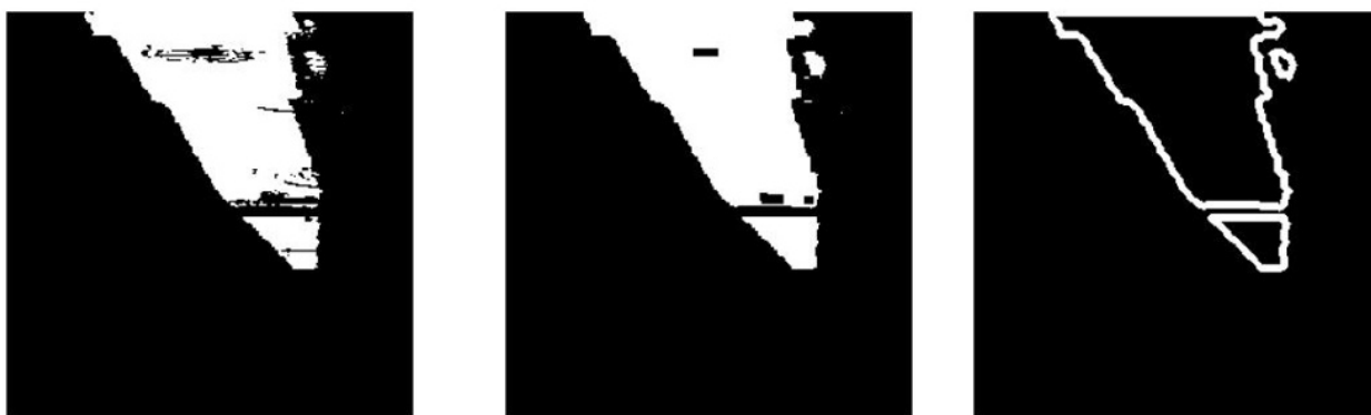
Figure 4.6: Example of the pre-processing pipeline applied to a short tip, showing the resized image after binarization (left), closing operation (center), and contour extraction (right).
