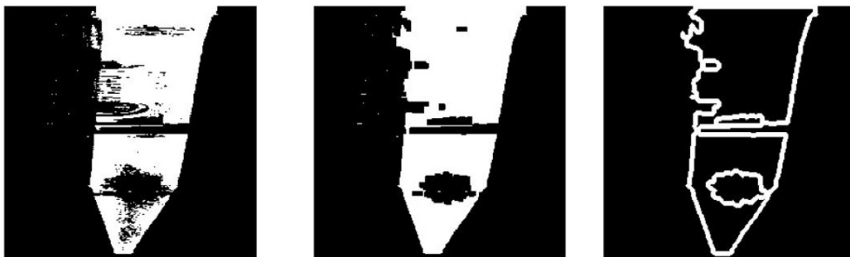
Figure 4.5: Example of the pre-processing pipeline applied to a long tip, showing the resized image after binarization (left), closing operation (center), and contour extraction (right).
