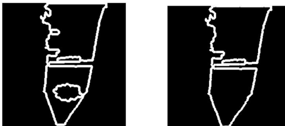
Figure 4.7: Example of a contour image obtained after pre-processing (left) and its corresponding reconstruction using the first 8 Fourier descriptors (right) for a long tip.
