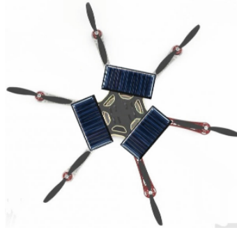
Fig. 2. Solar system power supply
