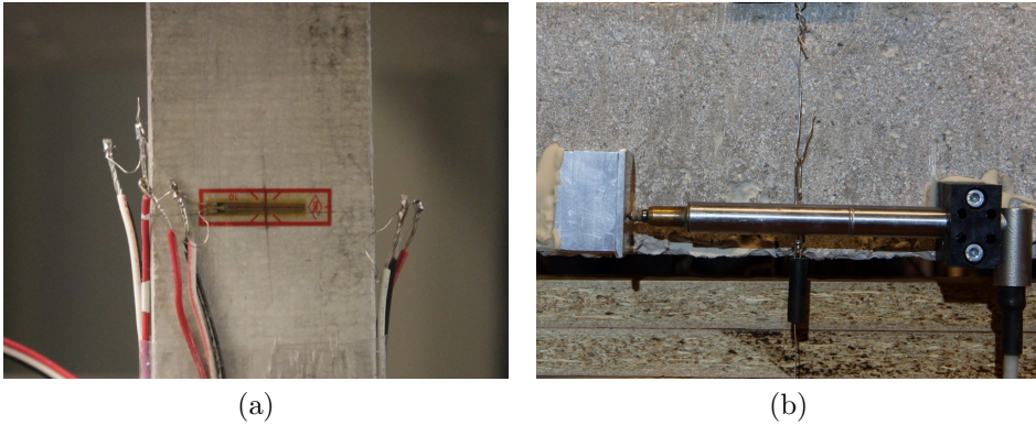
Fig. 2.2: Strain gauge (a) and LVDT (b)
