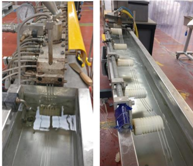
Figure 16 Extrudate exiting the die and passing the cooling bath
