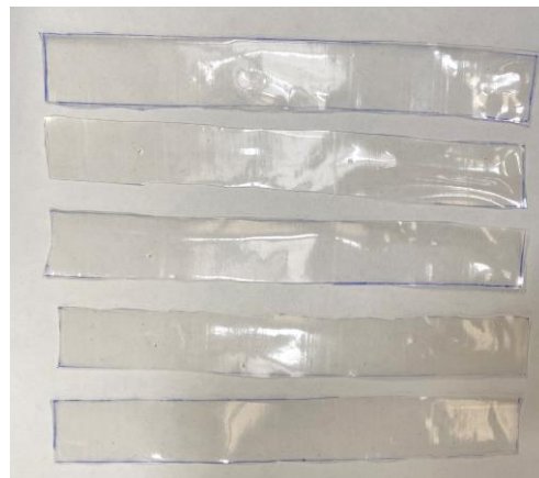
Figure 46 Standard sample dimension of film (PLA/ATBC – MD)
