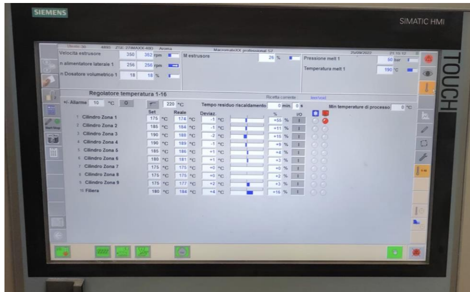
Figure 23 PLA/PHACT reactive extrusion parameters
