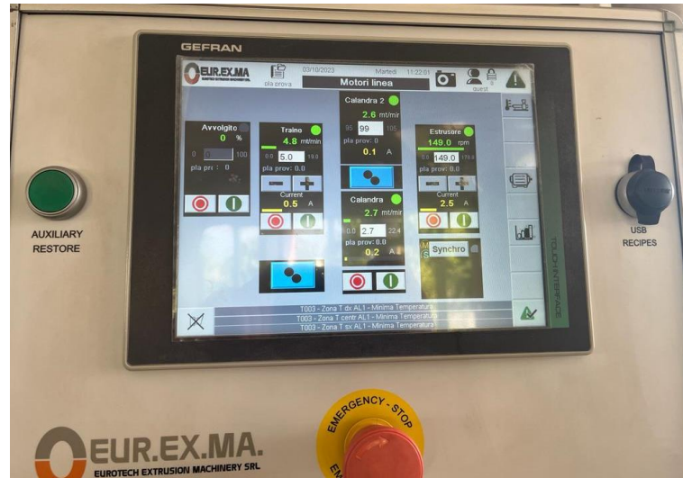
Figure 42 PLA/ATBC optimized cast parameters
