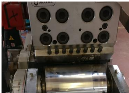
Figure 37 a) Cast extrusion die regulation, b) attaccapanni die
