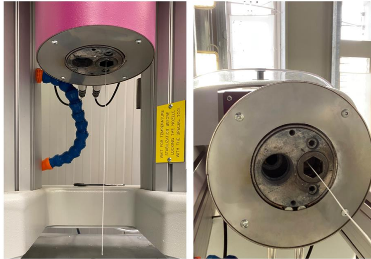
Figure 30 Compound PLA/PHACT melt flowing through the capillary mold
