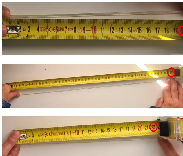
Figure 21 Qualitative tensile test on PLA/ATBC polymeric filament
