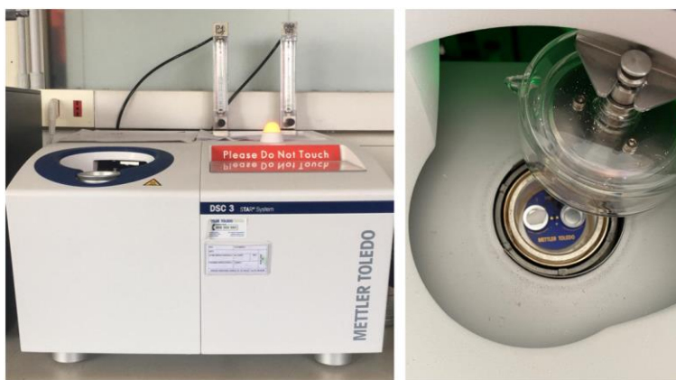
Figure 32 a) Mettler Toledo DS3 calorimeter, b) focus on the two crucibles
