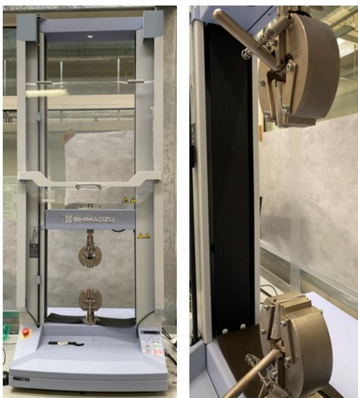
Figure 44 a) Shimadzu AGS-X universal testing machine b) standard specimen
