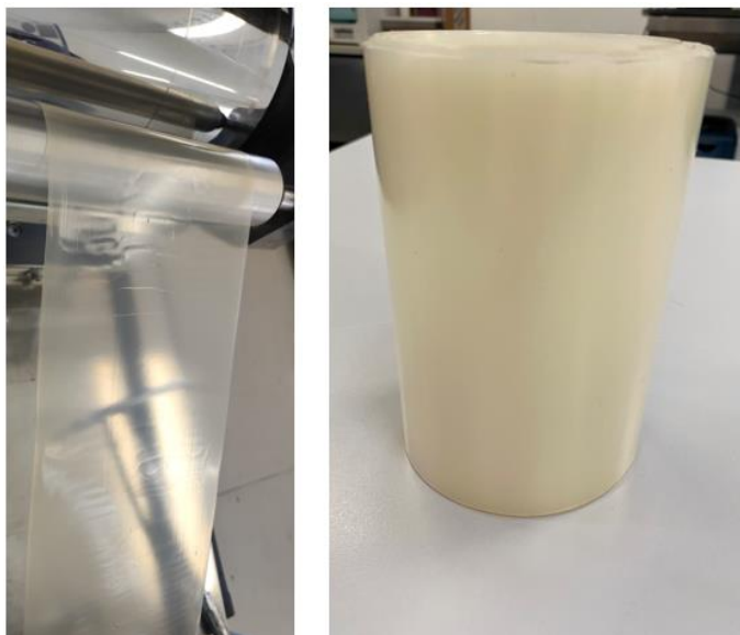
Figure 40 a) PLA/PHACT cast extrusion, b) PLA/PHACT film
