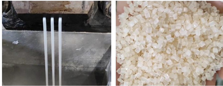
Figure 22 PLA/PHACT: a) extrudate, b) pellets
