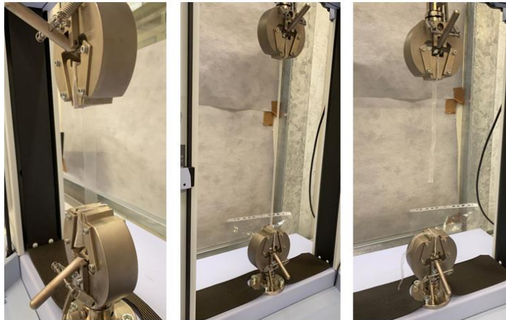
Figure 50 PLA/ATBC tensile test: a) start, b) elongation at break; c) after break
