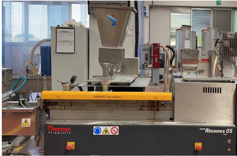
Figure 15 Twin screw extruder Haake Thermo Scientific Rheomex PTW 24MC Observing in the extrusion direction the Haake extruder (Figure 15), from right to left, the 10 sections of the barrel are designed to provide proper features:
