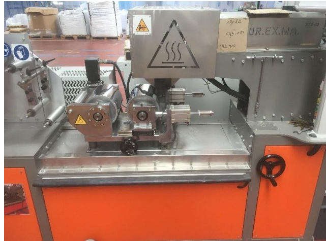
Figure 36 Lab-scale cast extruder Minicast 20
