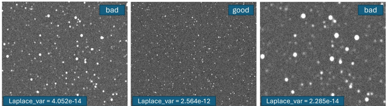
Figure 39. Three frames evaluated during the focusing routine: the left frame is in the intra-focal position, the right frame is in the extra-focal position, and the center frame shows the optimal Laplacian variance achieved at the end of focusing.
