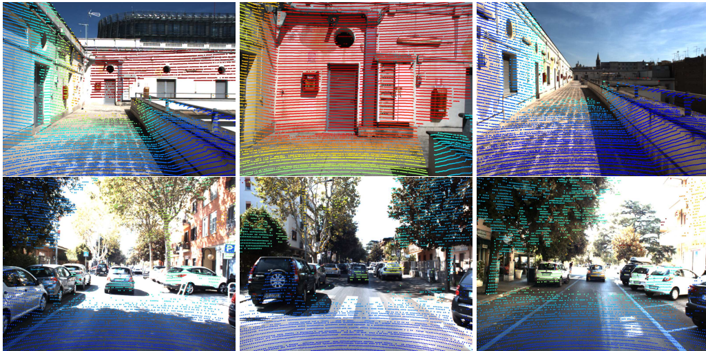
Figure 3.6. Qualitative examples of LiDAR cloud projection on RGB images. The recording setting is the one sketched in Fig. 3.4, where the parallax between the sensor is approximately 66 cm.
