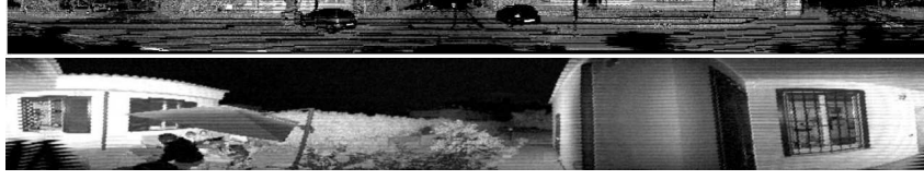
Figure 6.3. Spherical projection (described in Sec. 2.3.2) of the KITTI LiDAR points into an image plane (up) and of our LiDAR. Although deskewed, KITTI LiDAR sensor exhibit lower resolution compared to modern industrial-grade LiDARs.
