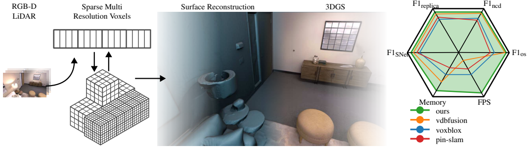
Figure 8.1. Overview. Our pipeline for real-time 3D reconstruction and rendering. Our variance-adaptive voxel grid dynamically adjusts resolution based on Truncated Signed Distance Function (TSDF) variance, enabling compact and accurate reconstructions from both RGB-D and unstructured 3D point cloud. The mesh output supports high-quality rendering via Gaussian Splatting, with adaptive splat control handled fully on the GPU.
