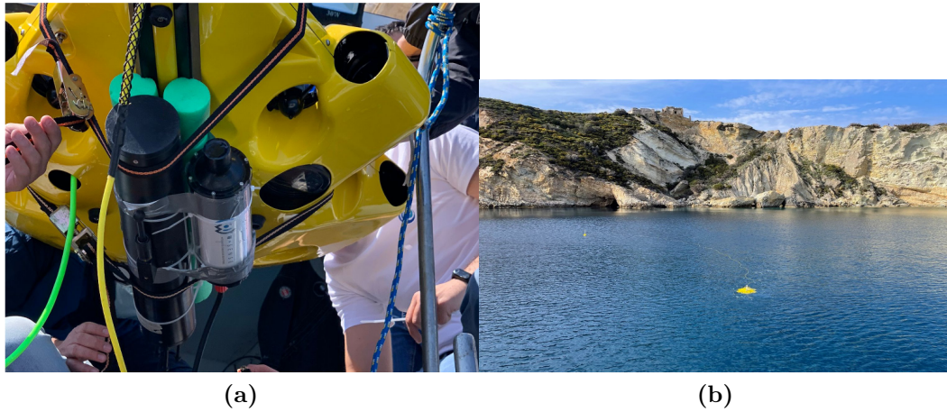
Figure 3.4. (a) WSense acoustic modem integrated in the hull of the Zeno AUV. (b) The Zeno AUV during navigation in the waters of Ponza.
