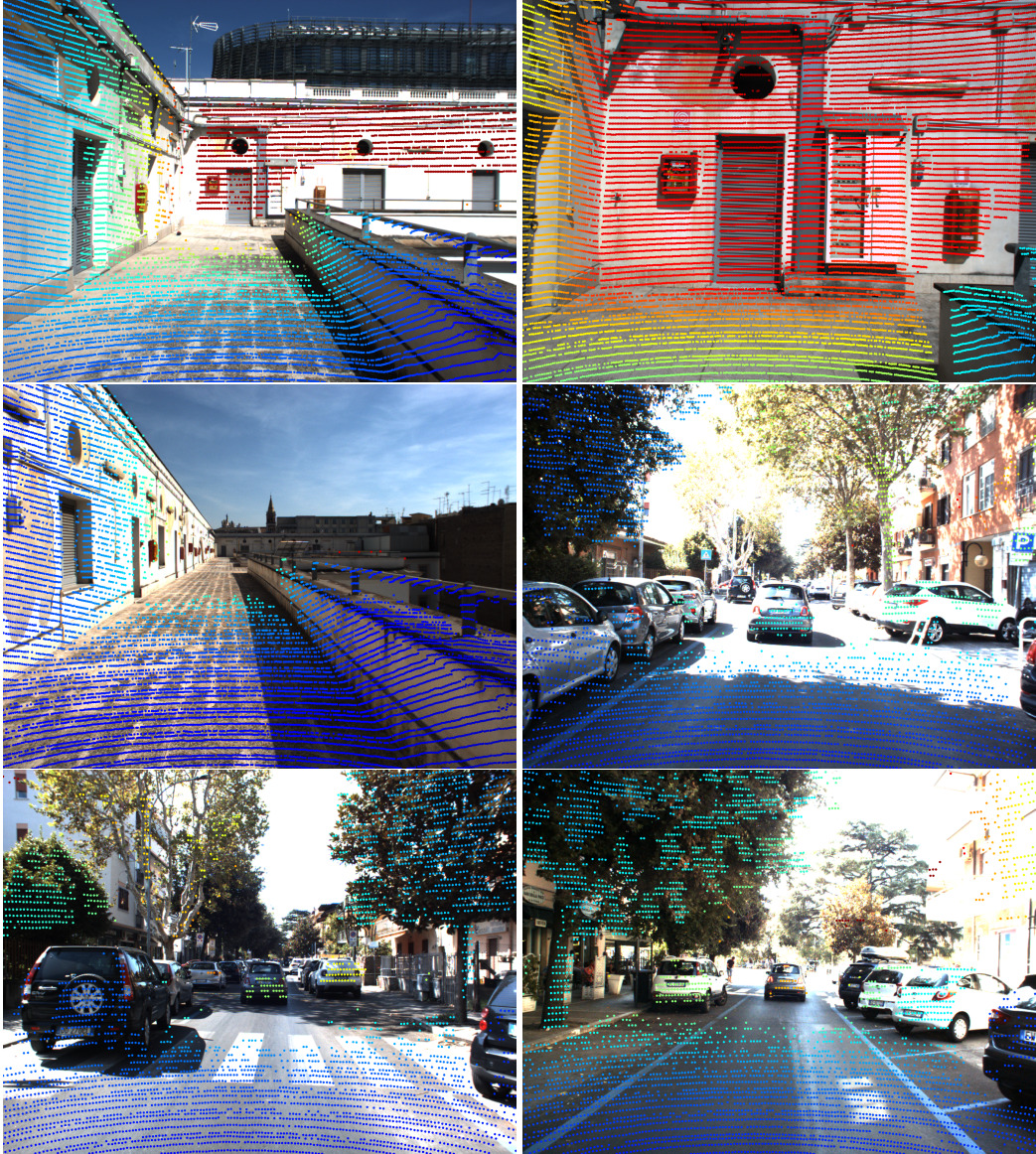
Figure 5.6. Qualitative samples showing L cloud projection on RGB image, in the setting sketched in Fig. 5.4, where the parallax between the sensor is approximately 66 cm.
