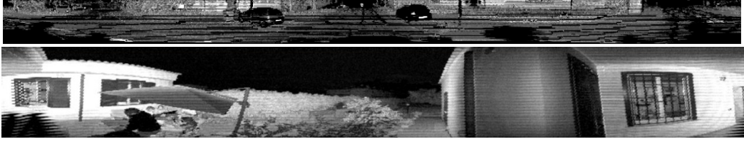
Figure 4.3. Projection of the KITTI LiDAR point cloud into an image plane (up), projection of our LiDAR into an image plane (down). The many holes of the up image due to uneven distribution of the LiDAR beams and calibration issues make the KITTI LiDAR image unusable for computer vision tasks.
