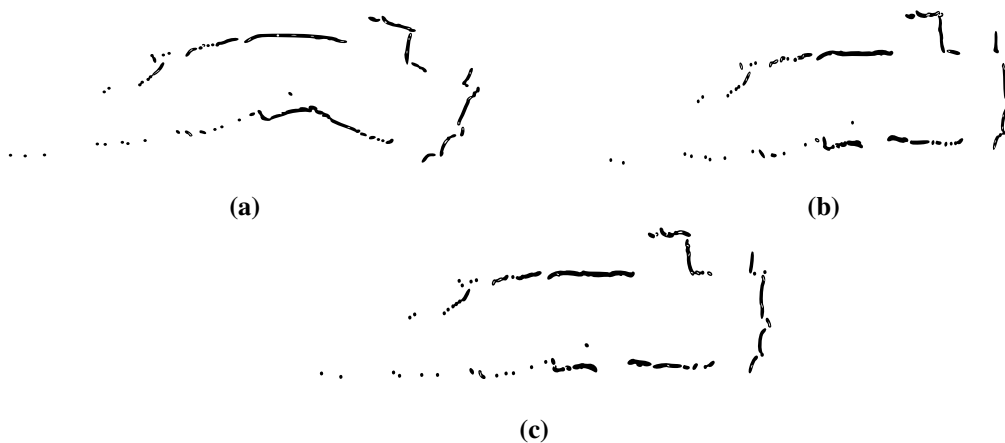
Figure 7.1. Effect of de-skewing. (a) Unprocessed (raw) scan acquired by a rotating robot, while (b) is the corresponding ground truth scan, and finally (c) is the same scan in (a), processed (de-skewed) using our proposed approach.
