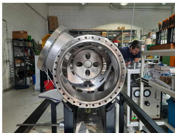
Figure 3.8: The "Basis" chamber for the project of PLD setup (photos were done at Ionvac S.R.L.(Pomezia, Lazio) during my internship
