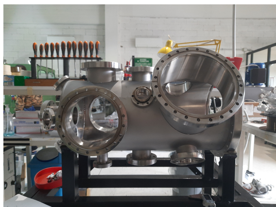
Figure 3.8: The "Basis" chamber for the project of PLD setup (photos were done at Ionvac S.R.L.(Pomezia, Lazio) during my internship
